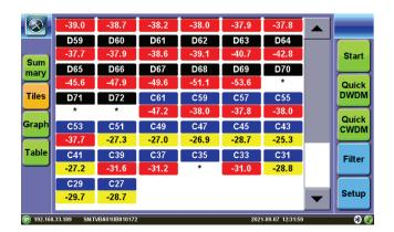
The power meter displays the current channel as well as the peak wavelength of that channel. It monitors the maximum and minimum composite power of that channel and takes the average of the power level and displays it in the center.
