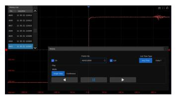
History function can record up to 170,000 frames of waveforms. The recording is executed automatically so that the customer can playback the history waveforms at any time to observe unusual events and quickly locate the area of interest using the cursors or measurements. The failed frames of the Mask Test can be stored as history
