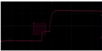
Zone Trigger is available for advanced triggering. Combine spatial triggering with common trigger modes to isolate signals of interest
