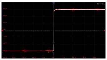
Segmented memory collection will store the waveform into multiple memory segments (up to 170,000) and each segment will store a triggered waveform as well the dead time information. The interval between segments can be as small as 1.5  $\mu$ s. All of the segments can be played back using the History function
