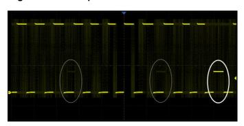
With a waveform update rate of up to 160,000 wfm/s, the oscilloscope can easily capture unusual or low-probability events. In Sequence mode, the waveform capture rate can reach 650,000 wfm/s
