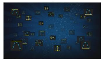
Parameter measurements include 4 categories: horizontal, vertical, miscellaneous, and CH delay providing a total of 60+ different types of measurements. Measurements can be performed within a specified gate period. Measurements on Math, Reference, and History frames are supported
