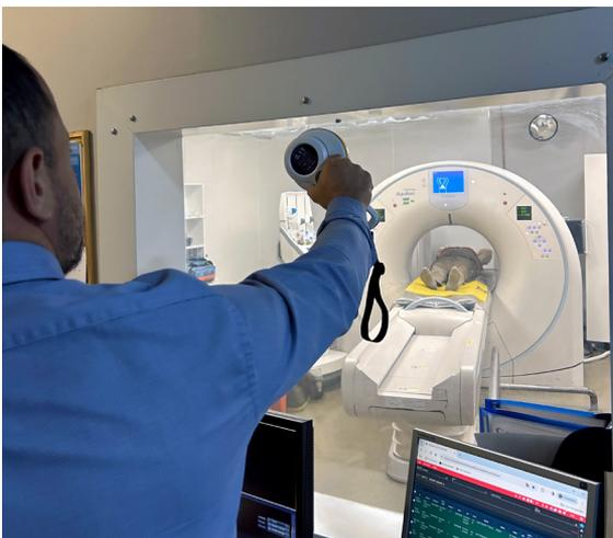
Figure 1: Survey meter used for detection of possible wall leakage from a room equipped with a CT machine.
