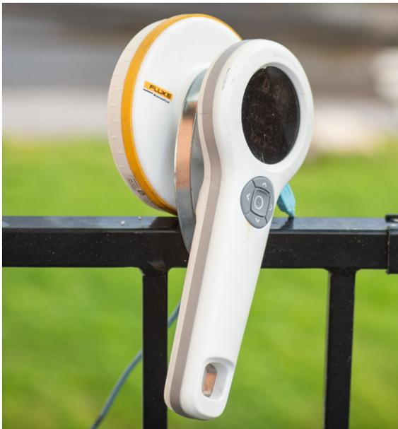
Figure 6: The RaySafe 452 survey meter was tested outdoors for approximately two and a half years, demonstrating its ability to withstand challenging environmental conditions, including summer heat, winter cold, rain, storms, and everything in between.
