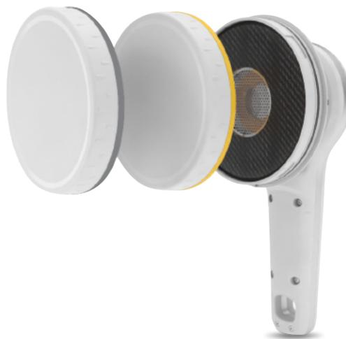
Figure 3: The active sensor area of the RaySafe 452 features a GM pancake detector behind a steel grid, encircled by a semiconductor detector consisting of a cluster of solid-state sensors under a carbon fiber cover. The full version of the RaySafe 452 includes two interchangeable lids: Ambient and Air Kerma. When either lid is mounted, the device measures dose and dose rate. Without a lid, it measures counts of  $\alpha$ ,  $\beta$ , and  $\gamma$  radiation.
