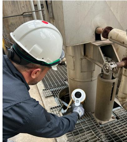
Figure 2: Survey meter used for control of a nuclear level gauge within the oil & gas industry.
